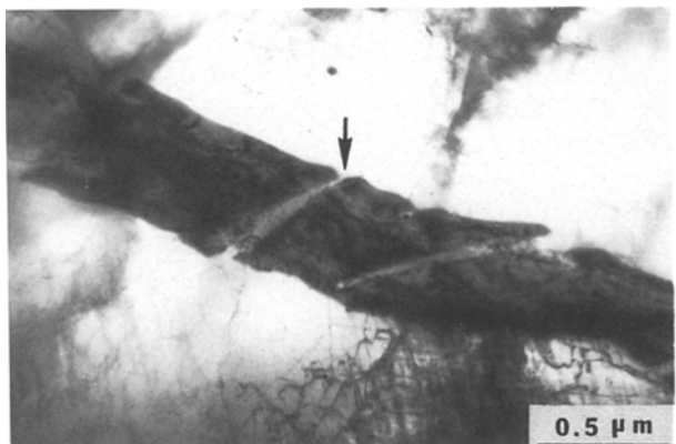
Figure 7 Thin-foil micrograph of temper rolled steel B. Note cracks in the cementite film.
